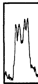
Fig. 2.—Fine structure of the allylic proton of compound IXb; J_1 \cong 2.5 cps., J_2 \cong 1.0 cps.
